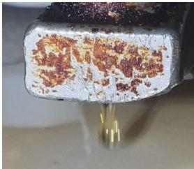
Damage is caused when operators engage the rear (magnet) end of the filter drain pan with the element lift tool, then drag the assembly across the floor. This action causes the plug and play end of the filter pan to tilt downward and contact the floor, causing excessive wear on the horizontal and vertical suction tubes until an oil leak occurs. It is best practice for operators to carry the filter drain pan instead of dragging.
